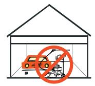
NEVER place pressure washer engines in garage, carport, or other enclosed space during use.
