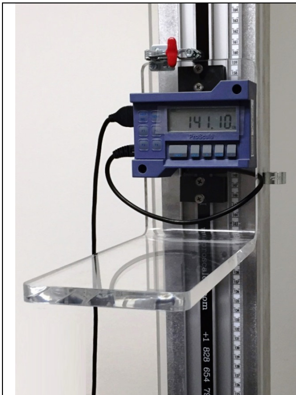
Exhibit 2-6. Stadiometer headpiece and digital measurement device
