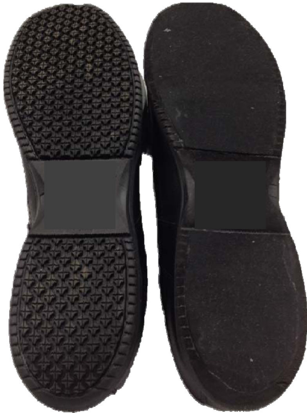
Figure 1. Picture of the fully treaded shoes (left) and the untreaded shoes that had the tread fully removed (right).
