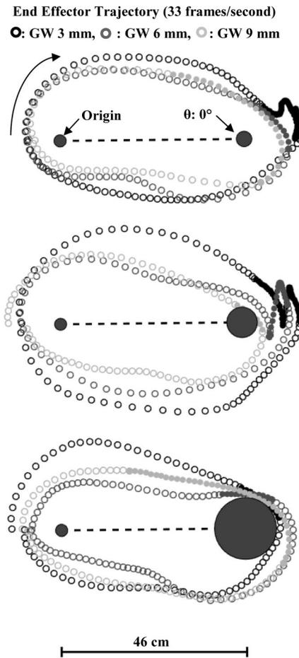
**Figure 4.** Sample participant data showing the end effector trajectory when threading a target pulley located at  $0^\circ$  (i.e., moving to a 3 o'clock position and back). Panels (from top to bottom) depict increase in pulley outer diameter (OD). Within each panel, data trajectories depict the influence of changing groove width (GW). The dwell phase for each trajectory is indicated by filled in circles.
