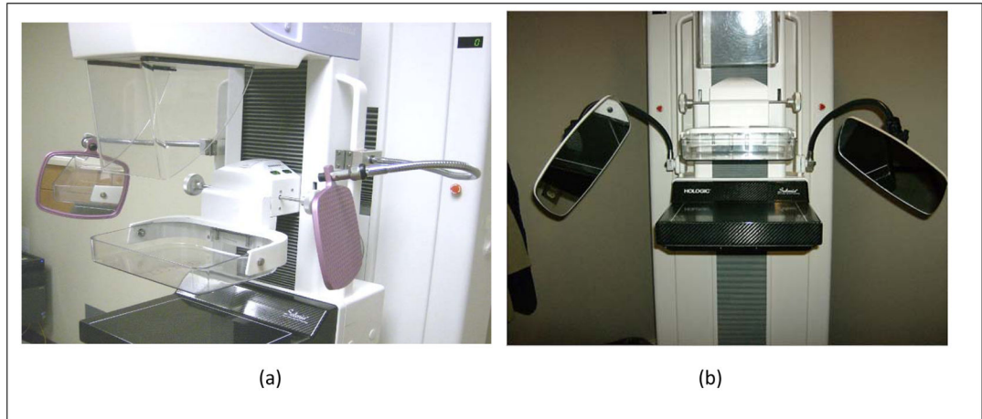
Figure 4. Prototype pair of mirrors used in the field study (a); design refinements seen in the system that is currently in use were based on field study experience (b).
