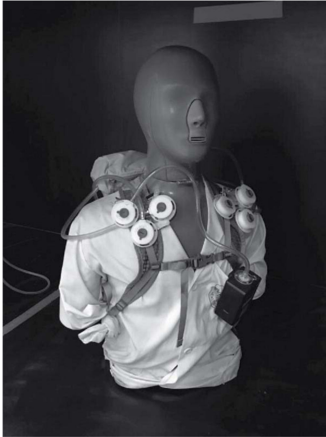
Figure 3. Mannequin equipped with six pump/sampler assemblies (three pumps at 2 L/min and three pumps at 10 L/min).
