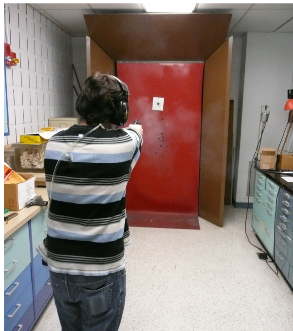
Figure 4. The firearms examiner fires a weapon into the bullet trap. The photo shows the visible cloud of airborne particles produced when firing.
