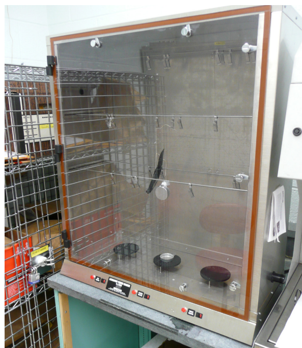
Figure 2. A super glue fuming chamber for fingerprint development with a suspended knife inside.
