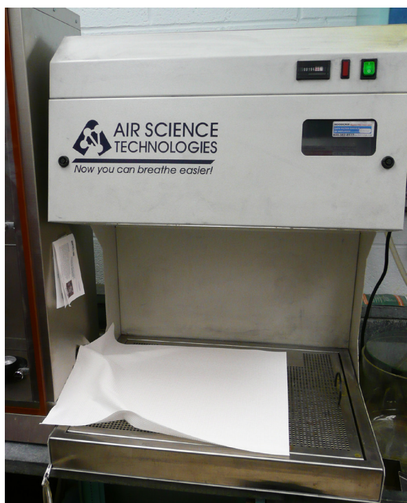
Figure 7. Ductless hood used during evacuation of vapors.
