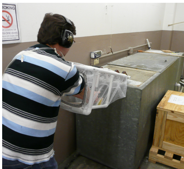
Figure 5. The firearms examiner fires a weapon into the water tank.
