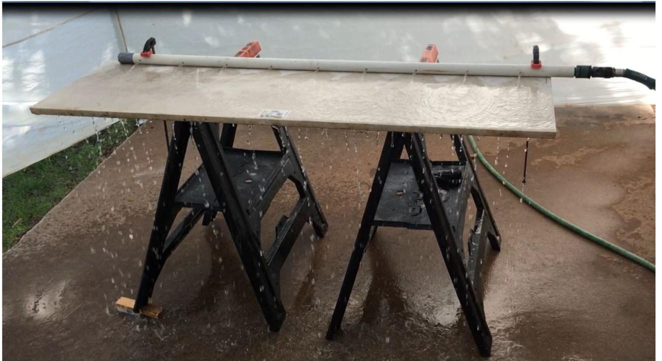
Figure 2. Experimental setup for wet operations using sheet flow wetting via a perforated water distribution manifold.
