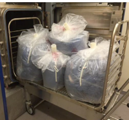
The autoclave process is used to inactivate laboratory waste before it's sent to the landfill.
