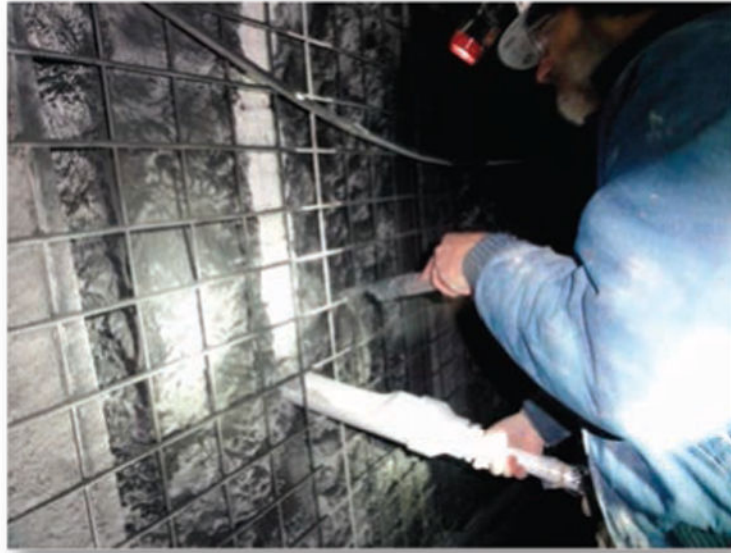
Figure 5. Rib dust collection using a plastic scoop and a 5-cm (2-in.)-wide narrow brush.
