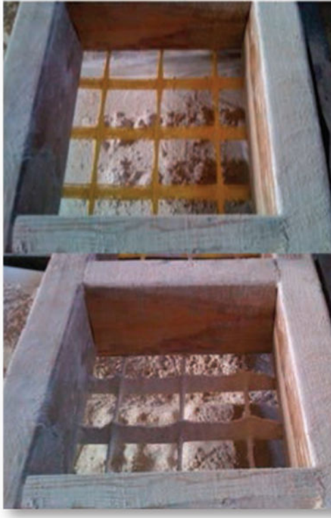
Figure 6. Small frame with Huesker 35/35 mesh before and after loading with rock dust.
