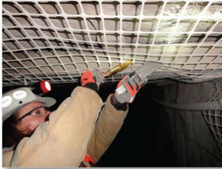
Figure 4. Dust collection from roof mesh using the MSHA pan-and-brush technique.
