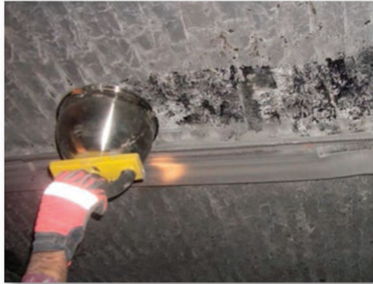
Figure 3. Using the bowl and brush to collect a roof dust sample in an underground coal mine.
