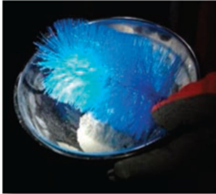
Figure 2. A long bristle brush in a bowl dust collector worked well as a collection method for dust on the roof and mesh.
