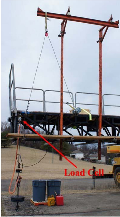
Figure 3. Dead-weight Drop Test Configuration
