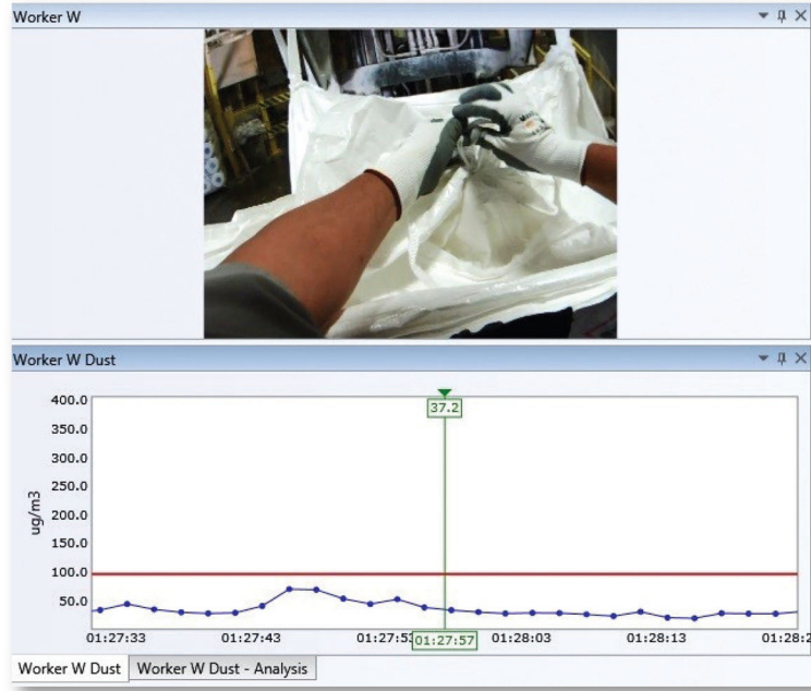
Figure 2. Bagging operator folding the bag’s loading collar to the side while tying his bulk bag.
