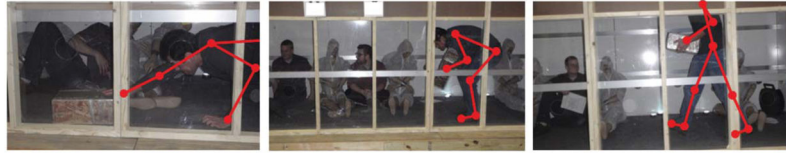
Figure 8. 0.6 m (24 in), 1.2 m (48 in), and 1.8 m (72 in) (left to right) mock-up heights for the move/carry portion of the ‘Changing of a CO 2 scrubber cartridge’ task.
