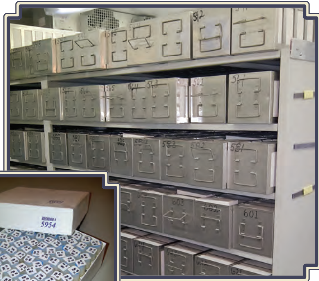
▲ Large racks in a -30° walk-in freezer hold the Specimen Bank samples. ▲ Plastic vials provide long-term protection and are bar-coded for rapid identification.
