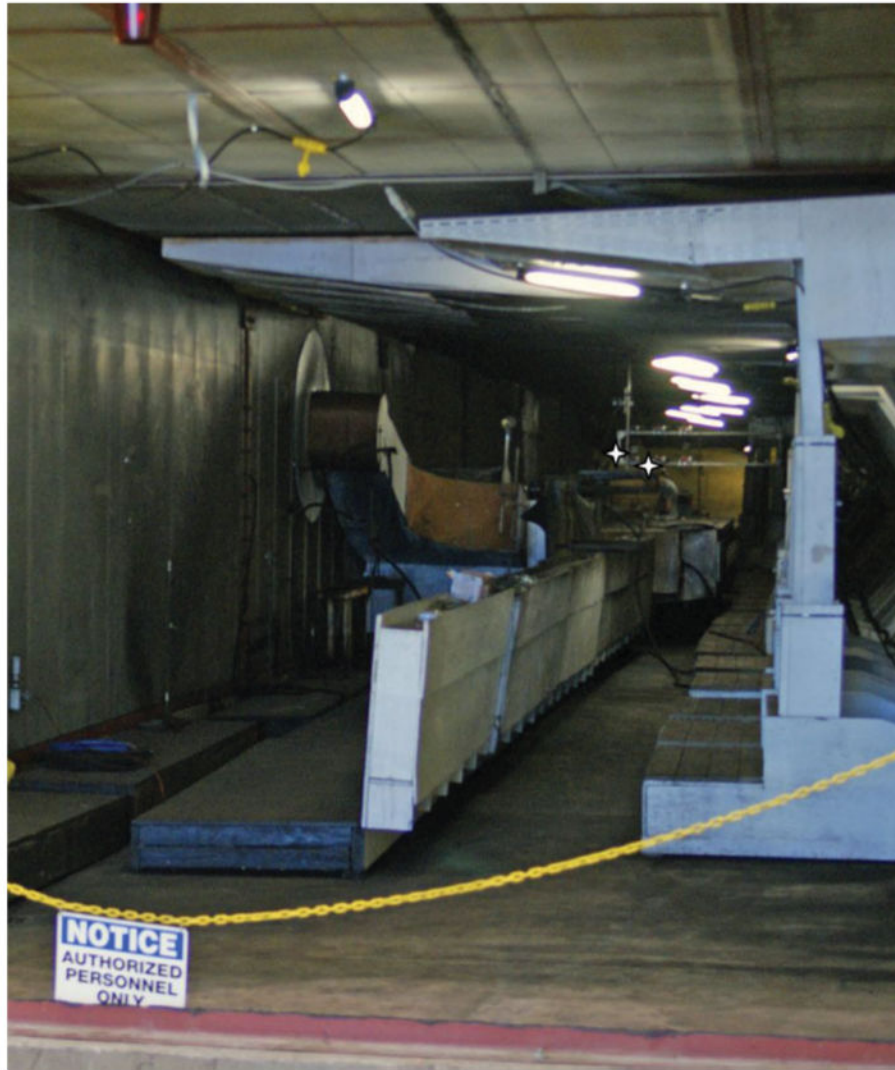
Figure 1. Longwall gallery used for the experiments. Toward the end of the gallery, the sampling rack can be seen, especially the alignment lasers (shown as white stars).
