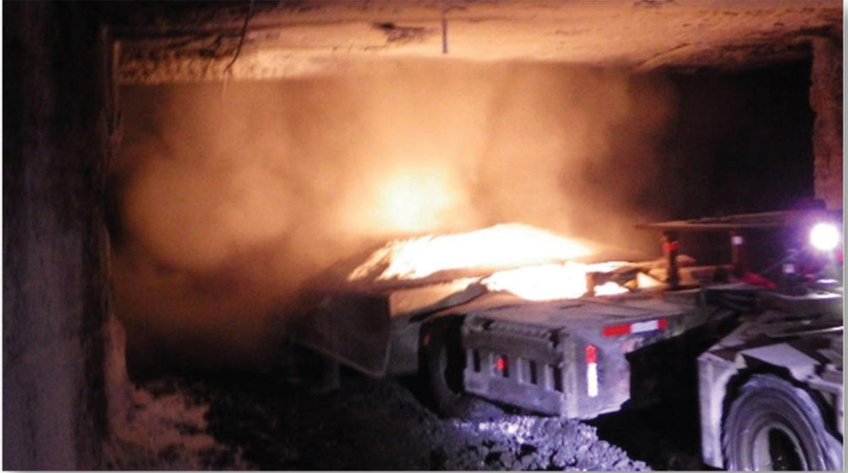
Figure 6. Flinger rock dusting machine applying the mine's dry rock dust.
