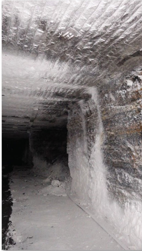
Figure 5. Moist rock dust applied to the mine entry by the flinger rock dusting machine.
