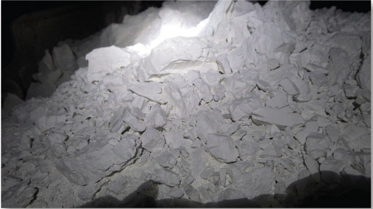
Figure 3. Untreated rock dust in the scoop. The rock dust is moist throughout.
