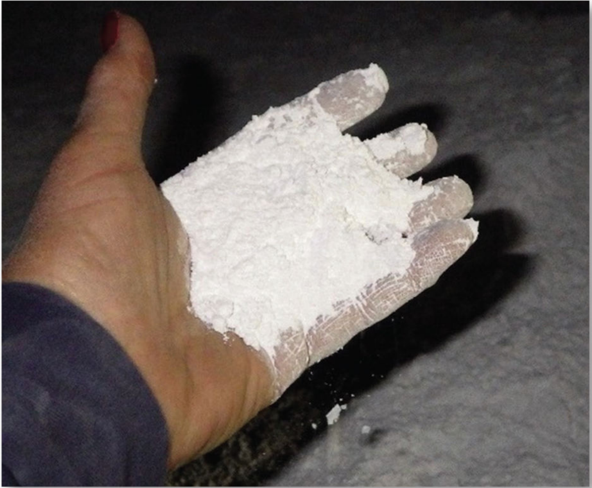
Figure 7. Treated rock dust, which was dry and fluffy when loaded into the scoop.
