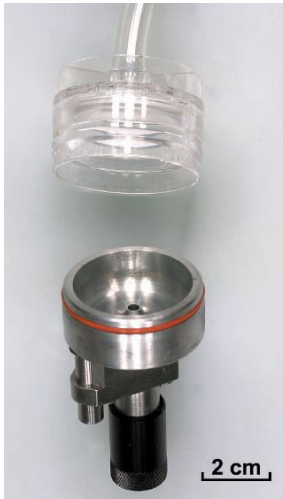
Figure 2H. Higgins-Dewell cyclone. This sampler was developed and used primarily as a respirable sampler in the UK. This version provides an interface directly to a 37-mm cassette. Cyclone construction is steel and operates at 2.2 L/min.
