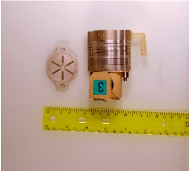
Figure 2J. Personal cascade impactor sampler (model Marple 290, Thermo Fisher Scientific). The sampler has five stages in the version shown and an additional three stages are available to provide cutpoints from 0.4 \mu\text{m} to 21 \mu\text{m} . The flap over the inlet reduces direct projection of large particles into the inlet. This sampler allows measurement of aerosol size distribution and calculation of respirable and thoracic fractions. It is constructed of aluminum and operates at 1.7 L/min.
