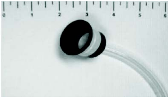
Figure 2F. Bell mouth cowl sampler. An alternative to the standard asbestos sampling cassette. The inlet is flared to reduce the effect of external air motion on sample uniformity. It is made of conductive plastic and is operated at a flow rate between 0.5 L/min to 16 L/min.
