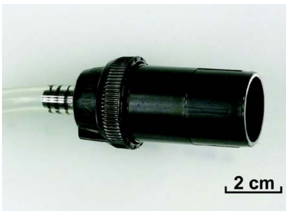
Figure 2E. Asbestos sampling cassette. The long (50 mm) inlet was designed to prevent incidental contact with the filter surface and, when facing downward, acts to a certain extent as an elutriator, preventing larger particles from reaching the filter surface. It is made of conductive plastic and is operated at a flow rate between 0.5 L/min to 16 L/min.
