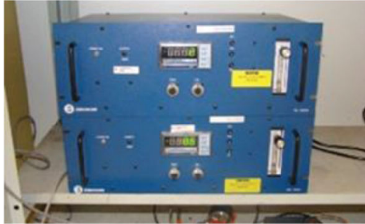
Figure 4. CO and CO 2 IR gas analyzers.
