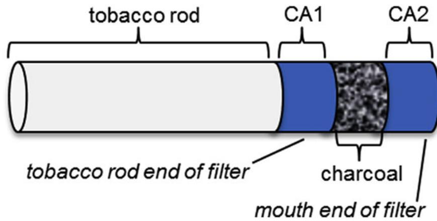
**Fig. 2.** Schematic overview of modified cigarette design. Cellulose acetate plugs (CA1 and CA2) are of equal lengths. Nonporous tape (not pictured) is wrapped around entire filter construct to contain charcoal and block any ventilation holes.
