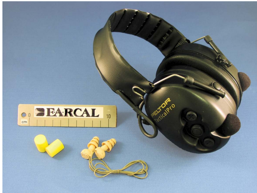
Figure 1. Measured hearing protection devices. 3M™ E-A-R™ Classic™ Earplug (foam earplug, left), 3M™ Combat Arms™ Single-Ended Earplug (level-dependent earplug, center), and 3M™ PELTOR™ TacticalPro™ Electronic Headset (electronic earmuff, right).
