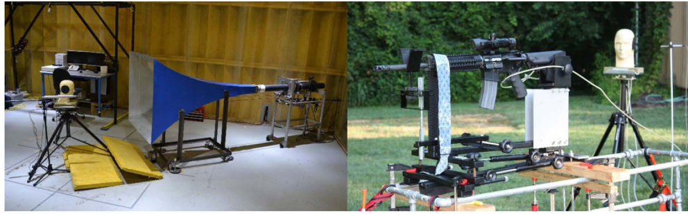
Figure 2. Experimental setups. Left: Acoustic shock tube and horn with ATF and blast probe microphone positioned in front of the horn in a hemi-anechoic chamber. Right: AR-15 with ATF and free-field microphone positioned for measurements at the 150 dB peak level.
