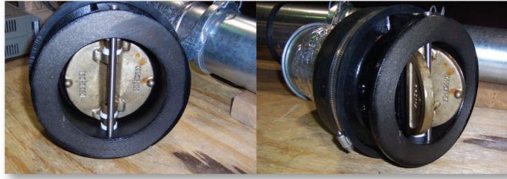
Figure 5. Brass/cast-iron butterfly check valve.
