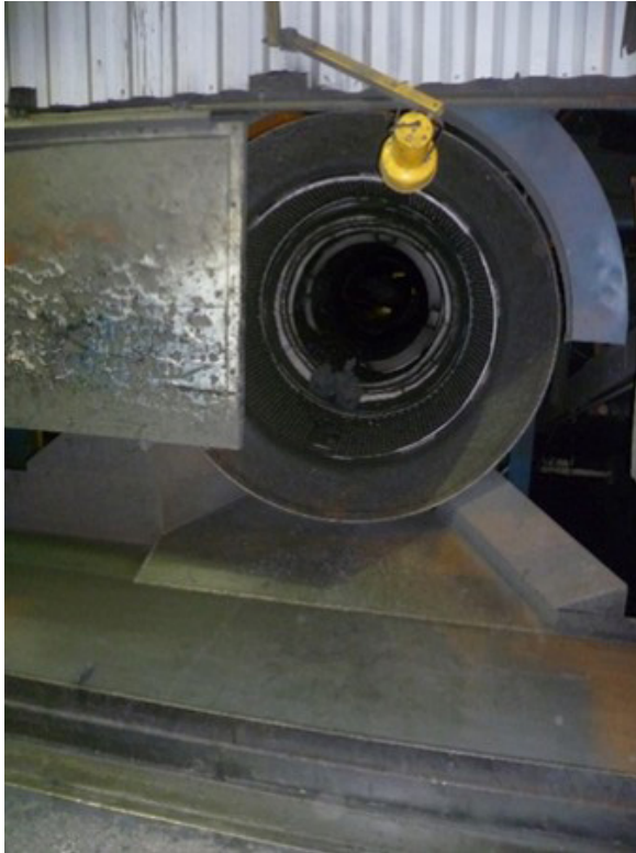
Figure 9. Barrier at exit of Didion roller. Photo by NIOSH.
