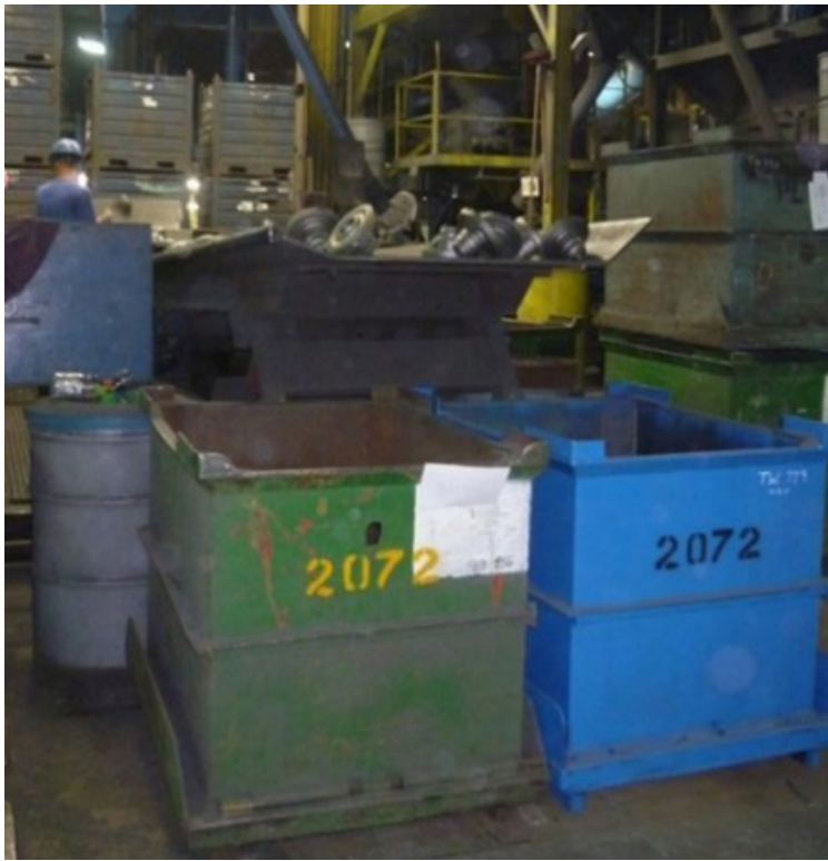
Figure 6. Metal castings dropping from end of shaker conveyor into two metal bins. Photo by NIOSH.
