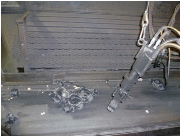
Figure 1. Hydraulic wedge suspended at one of the shaker conveyors. Photo by NIOSH.
