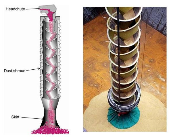
Figure 7.5. Cascade loading spout.
