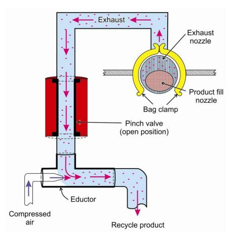
Figure 6.10. Dual-nozzle bagging system design.
