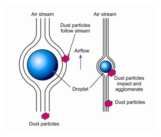
Figure 2.2. Effect of droplet size on dust particle impingement.
