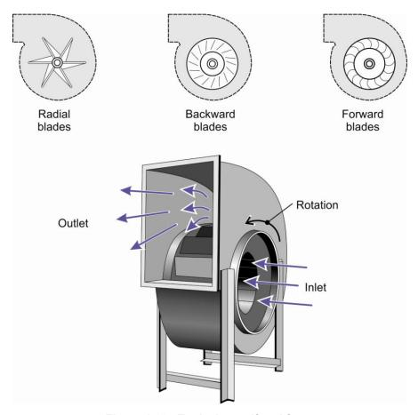
Figure 1.30. Typical centrifugal fan.
