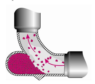
Figure 5.22. HammerTek wear-resistant elbow installed in conveying ductwork.
