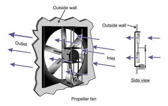
Figure 1.28. Wall-mounted propeller fan.
