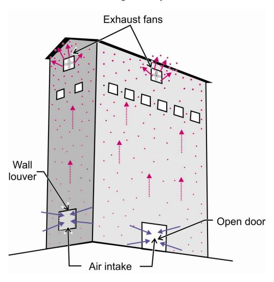
Figure 8.7. Basic design of total structure ventilation system.
