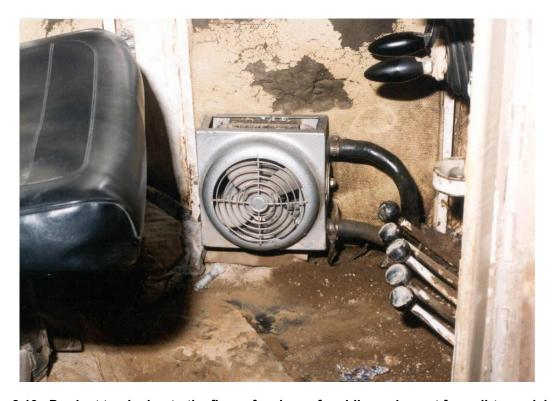
Figure 8.13. Product tracked onto the floor of a piece of mobile equipment from dirty work boots.
