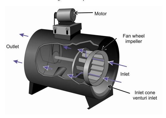
Figure 1.31. Axial centrifugal fan showing airflow [adapted from Bleier 1998].
