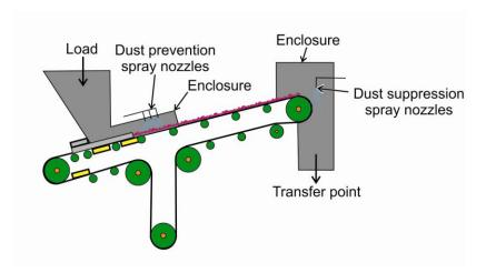
Figure 2.11. Typical conveyor dust control application.
