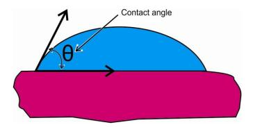
Figure 2.3. Contact angle resulting from a liquid meeting a solid surface [NDT 2009].
