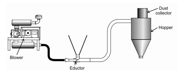
Figure 5.24. Conveyance system utilizing a venturi eductor device.
