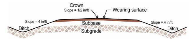
Figure 10.2. Cross section of haul road.
