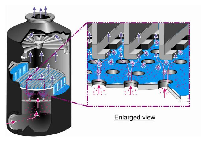
Figure 1.23. Typical design of an impingement plate scrubber.
