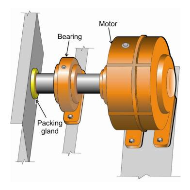
Figure 5.18. Packing gland and pillow block support bearing.
