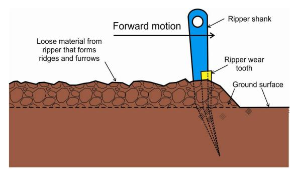
Figure 10.11. Example of tillage (from chisel plowing, for example) exposing large clods.
