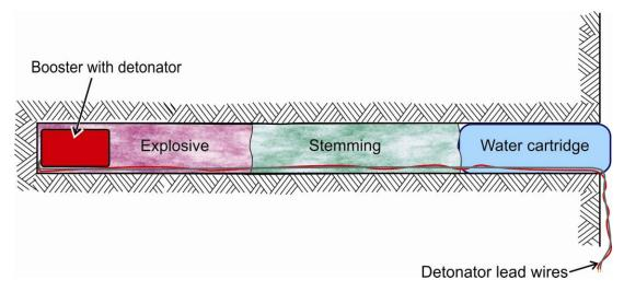
Figure 3.20. A typical blasthole containing an explosive charge utilizing a water cartridge to suppress dust generated during blasting.
