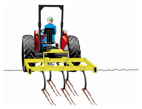
Figure 10.10. Chisel plow used for creating large clods in open areas to reduce wind erosion.
