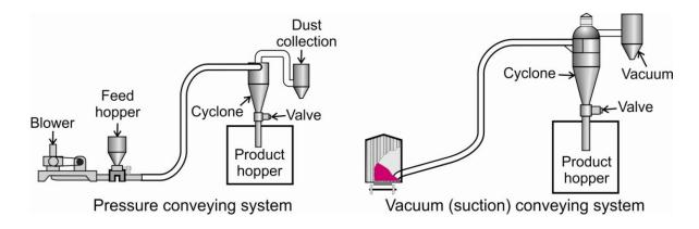
Figure 5.21. Depiction of two types of pneumatic conveying systems.
