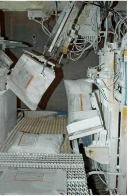
Figure 6.13. Bag storage shelves shown on left; a robotic arm with suction cups to place empty bags on fill nozzle shown on right.
