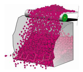
Figure 5.16. Typical impact bed designed for ore-on-ore contact at transfer locations or chutes.
