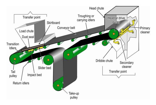
Figure 5.1. Basic components of a conveyor belt.
