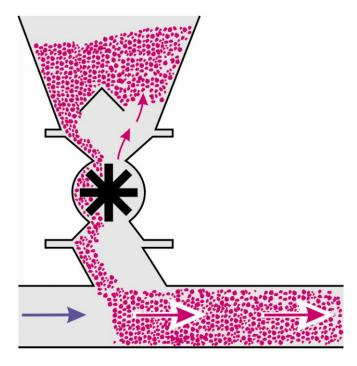
Figure 5.23. Rotary airlock feeding pneumatic conveying line.
