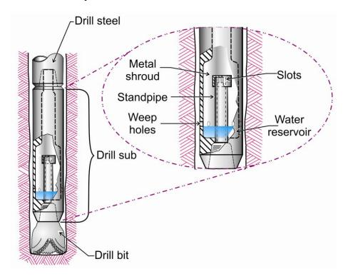
Figure 3.3. Internal workings of a water separator sub.
