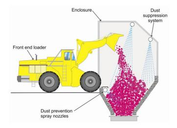
Figure 2.10. Typical loader dump dust control application.
