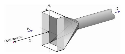
Figure 1.7. Hood entry loss calculation [adapted from ACGIH 2010].
