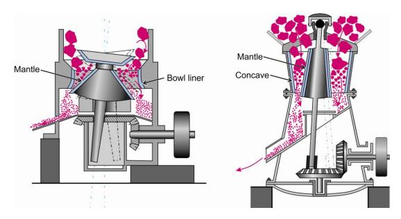
Figure 4.2. Examples of compressive crushers. Left—illustration of a cone crusher showing material being crushed between the cone mantle and bowl liner. Right—illustration of a gyratory crusher with material being crushed between the gyratory head and the frame concave.
