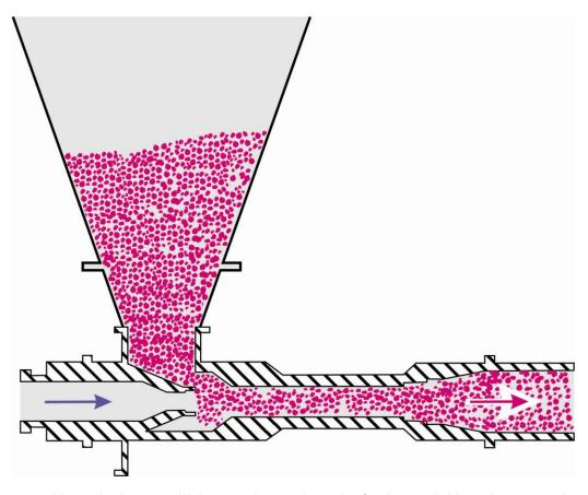
Figure 5.25. Venturi eductor utilizing suction to draw the feed material into the conveying line.
