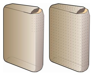
Figure 6.3. Undervalve bag perforations (left) and overall perforations (right).
