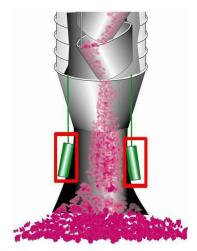
Figure 7.4. Skirt (in yellow box) and tilt sensors (in red boxes) installed on the discharge end of loading spouts to help reduce dust emissions.
