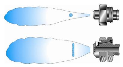
Figure 2.5. Typical air atomizing nozzle round spray pattern (top) and fan spray pattern (bottom).
