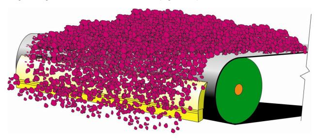
Figure 5.12. Typical method for scraping material from a belt.
