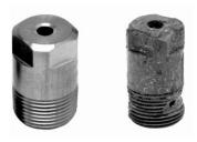
Figure 2.18. Temperature damage—new versus used [SSCO 2004].
