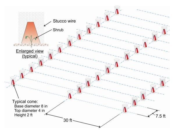
Figure 10.17. Layout demonstrating dispersed wind barriers.
