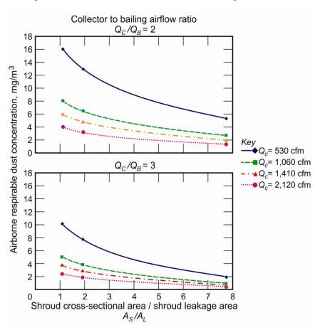
Figure 3.8. Graphs of the model that represents the severity of dust emissions based upon collector to bailing airflow ratios, showing that the respirable dust concentrations become lower as the collector to bailing airflow ratio increases.
