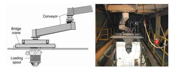
Figure 7.3. Articulated loading spout positioner.
