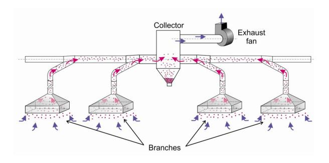
Figure 1.25. Demonstration of how a complex exhaust system is a combination of branches linking simple exhaust systems [adapted from ACGIH 2010].
