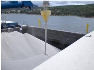
Figure 7.6. Dust Suppression Hopper creating a solid stream of material during loading to reduce dust liberation.
