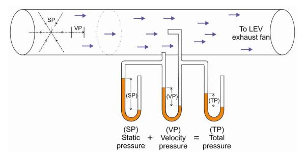
Figure 1.1. Relationship between static, velocity, and total pressure [adapted from ACGIH 2010].
