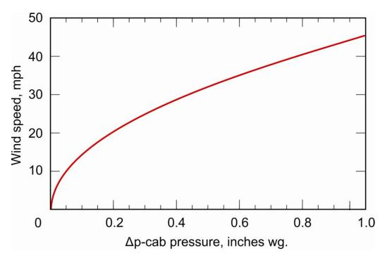
Figure 9.3. Positive cab pressure necessary to prevent dust-laden air from infiltrating the enclosed cab at various wind velocities.
