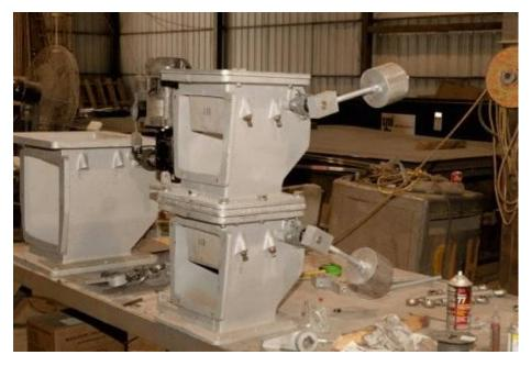
Figure 1.24. Double dump weight-based valves.
