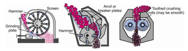
Figure 4.3. Examples of impactive crushers. Left—a hammermill-type crusher showing material crushed between the rotating hammers and fixed grinding plate. Center—illustration of material being crushed between rotating hammers and fixed anvil plates in an impact breaker. Right—illustration of the size reduction action of a roll crusher.
