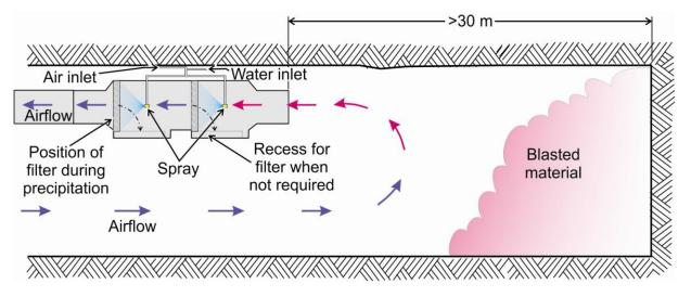
Figure 3.23. A filtration unit, located in the blast heading, used for filtering the contaminated ventilation air from the blast heading after blasting occurs.
