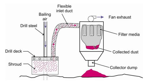
Figure 3.4. A basic dry dust collection system on a drill.
