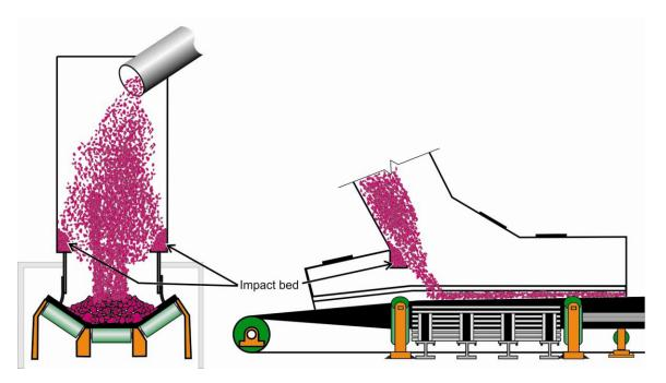
Figure 5.4. Depiction of impact bed used to control material direction and speed.
