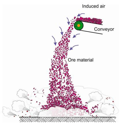
Figure 1.6. Demonstration of air induction as material falls from a conveyor.
