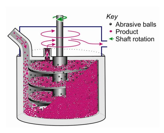
Figure 4.13. Illustration of a stirring mill.
