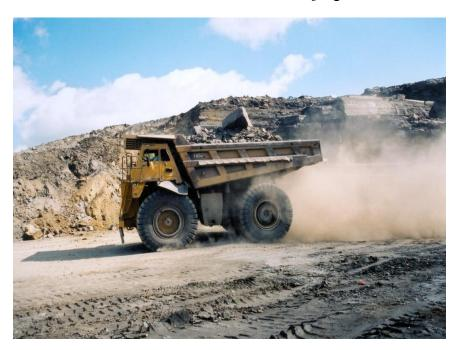
Figure 10.1. Example of haul road dust from a typical mine haul truck.
