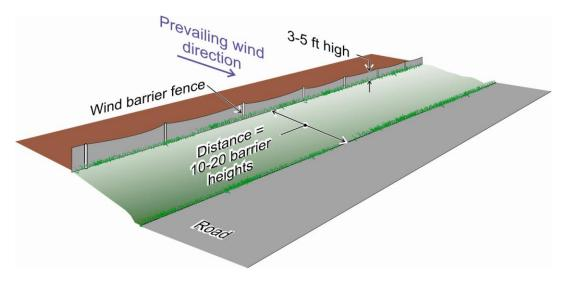
Figure 10.15. Demonstration of how fences are used as wind barriers.
