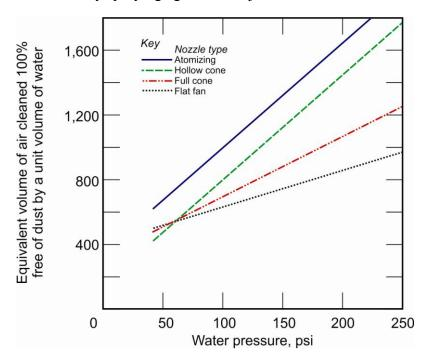
Figure 2.12. Airborne suppression performance of four types of spray nozzles [NIOSH 2003]. Atomizing nozzle is air atomizing, and hollow cone, full cone, and flat fan spray nozzles are hydraulically atomizing.
