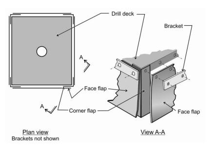
Figure 3.5. Reinforcing flaps added to each corner of a rectangular deck shroud to reduce leakage.
