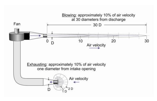
Figure 1.3. Comparison of ventilation characteristics for blowing versus exhausting system [adapted from Hartman et al. 1997].
