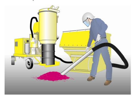
Figure 8.6. Portable system used to perform vacuuming.
