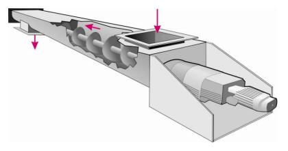
Figure 5.17. Depiction of a typical screw conveyor.
