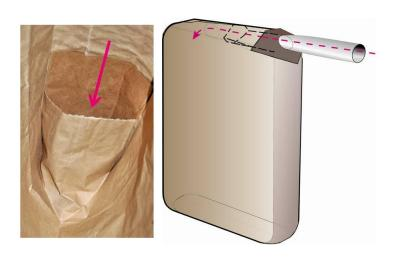
Figure 6.2. Typical bag valve—interior view (left). Artist concept of fill nozzle and bag valve (right). Fill nozzle enters through the bag valve and delivers product into bag.
