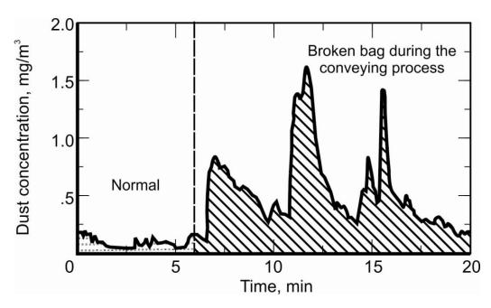
Figure 8.12. Increase in worker's respirable dust exposure from broken bag during the conveying process.
