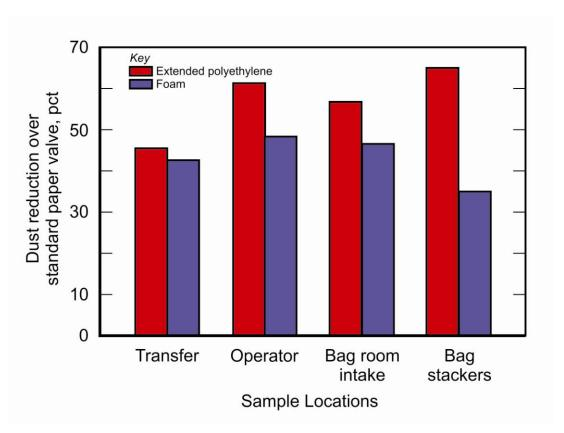
Figure 6.7. Dust reductions with extended polyethylene and foam valves as compared with the use of the standard paper valve.
