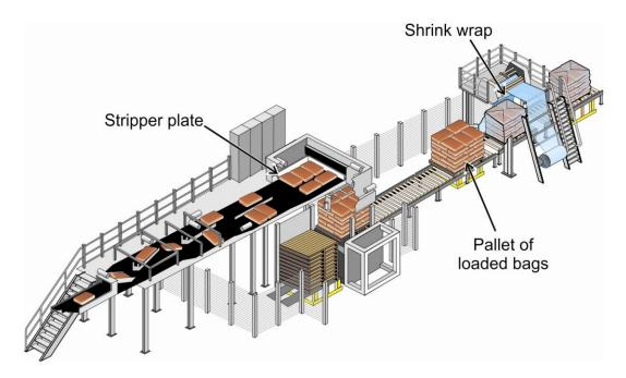
Figure 6.17. Figure of the automated high-level palletizing process.
