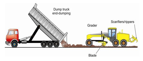
Figure 10.4. Use of end-dumping with grader to lay gravel onto road surface.
