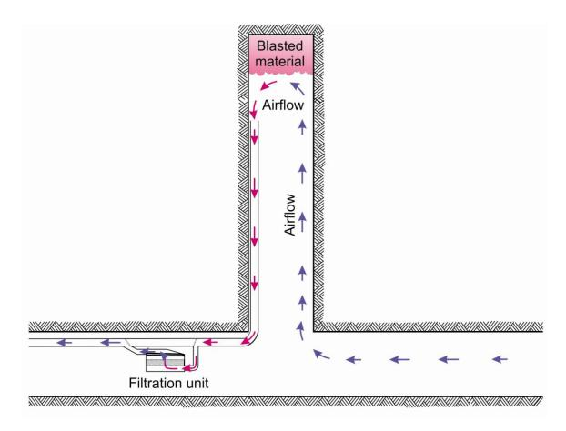
Figure 3.22. A filtration unit, located adjacent to the blast heading, used for filtering the contaminated ventilation air from the blast heading after blasting occurs.
