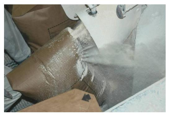
Figure 6.4. Undervalve perforations relieve excess pressure from bag during filling process to minimize the possibility of bag failure.
