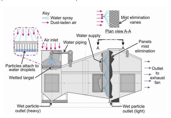
Figure 1.21. Typical design of a wet scrubber dust collector.
