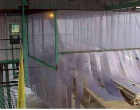
Figure 7.7. Rail car loadout area enclosed with plastic strips to contain dust.
