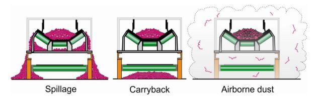
Figure 5.2. Types of fugitive dust emissions from conveyor belts.
