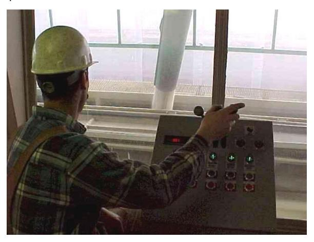
Figure 7.8. Environmentally controlled operator's booth near loadout area.
