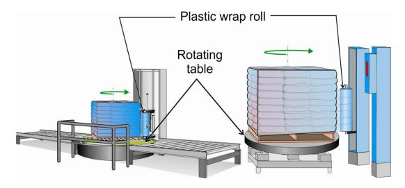
Figure 6.19. Automated spiral stretch wrap machine.
