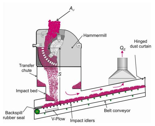
Figure 4.9. Illustration of a dry (exhaust) dust control system at the discharge of a hammermill crusher onto a belt conveyor.
