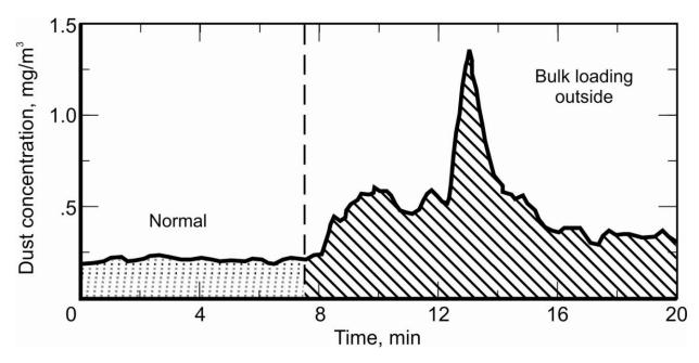
Figure 8.9. Increase in a worker's respirable dust exposure inside a mineral processing facility while bulk loading was being performed outside.
