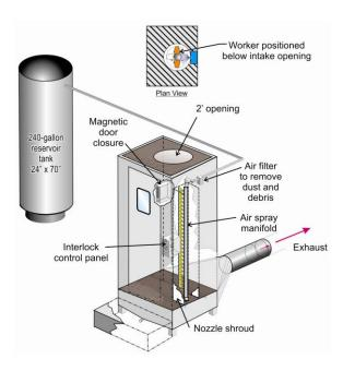
Figure 8.1. Design of clothes cleaning system.
