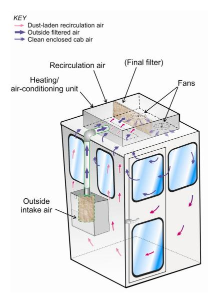
Figure 9.1. General design of an effective filtration and pressurization system.
