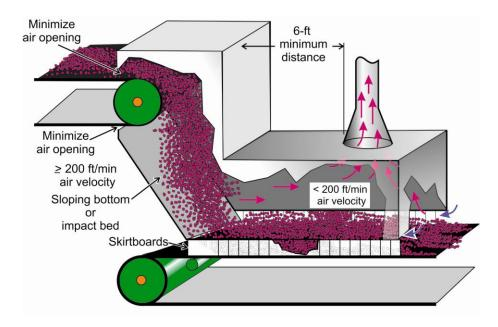
Figure 5.15. Conveyor transfer enclosure used with an exhaust ventilation system.
