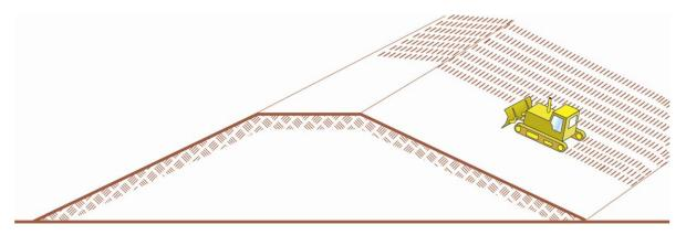
Figure 10.13. Dozer being used to compact stockpile for long-term storage.
