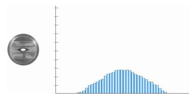
Figure 2.20. Good spray tip showing pattern and distribution graph [Schick 2006]. Height of bar indicates distribution of water over pattern width and indicates relatively uniform flow over the width of the pattern.
