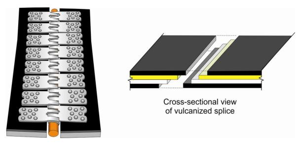
Figure 5.14. Illustration of a mechanical belt splice (left) and a vulcanized belt splice (right).
