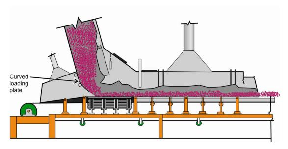
Figure 5.5. Depiction of curved loading plate to help steer loaded material in a particular direction.
