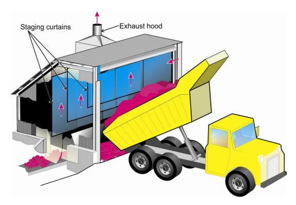
Figure 4.5. Illustration of a dry (exhaust) dust control system with a partial enclosure at a crusher dump loading operation.
