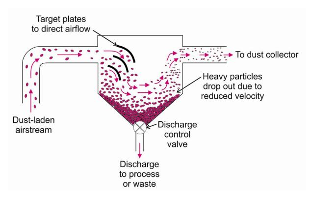
Figure 1.14. Typical design of gravity separator (drop-out box).
