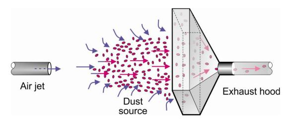
Figure 1.4. Simple design of basic push-pull ventilation system.
