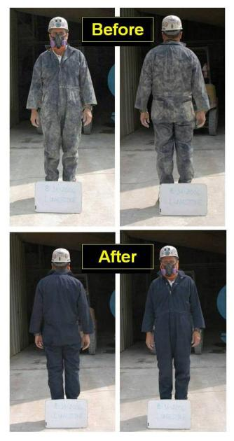
Figure 8.3. Test subject wearing polyester/cotton blend coveralls before and after using the clothes cleaning booth.
