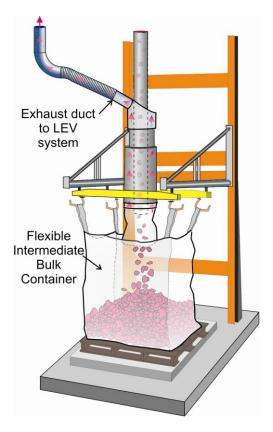
Figure 6.21. Exhaust ventilation system used during loading of Flexible Intermediate Bulk Containers.
