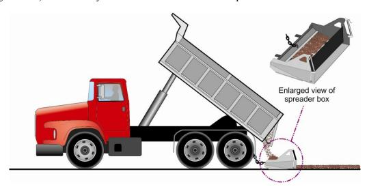
Figure 10.3. Use of a spreader box to lay gravel onto road surface.
