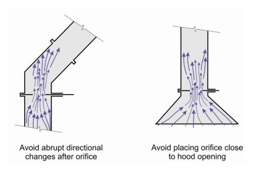
Figure 1.12. Demonstration of poor orifice plate placement.
