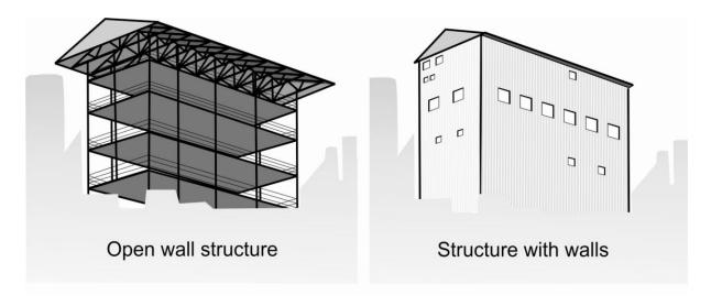
Figure 8.8. Open-structure design compared to standard walled structure.
