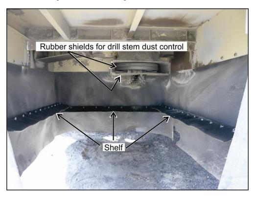
Figure 3.10. Air-blocking shelf installed on the inside perimeter of the drill shroud of a blasthole drill. Note the overlap in the rear corners to eliminate any gaps in the shelf perimeter.
