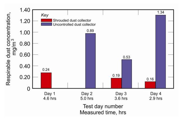
Figure 3.14. Comparison of dust concentrations of uncontrolled dust collector dump to shrouded dust collector dump.
