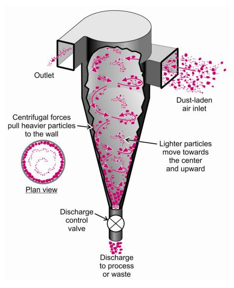
Figure 1.15. Typical design of a cyclone dust collector.
