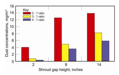
Figure 3.7. Results of changing dust collector to bailing air ratio at various shroud gap heights.
