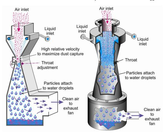
Figure 1.22. Typical designs of a venturi scrubber.
