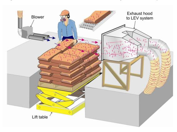
Figure 6.15. Semi-automated bag palletizing system to ergonomically improve bag stacking process with a push-pull ventilation system used to capture the dust generated.
