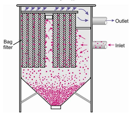
Figure 1.16. Basic design of a baghouse dust collector.
