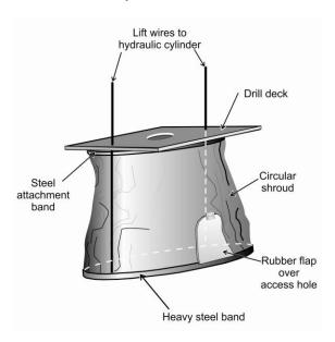
Figure 3.6. Circular shroud design.
