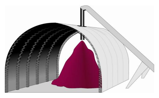
Figure 10.16. Barrier built to enclose a stockpile.
