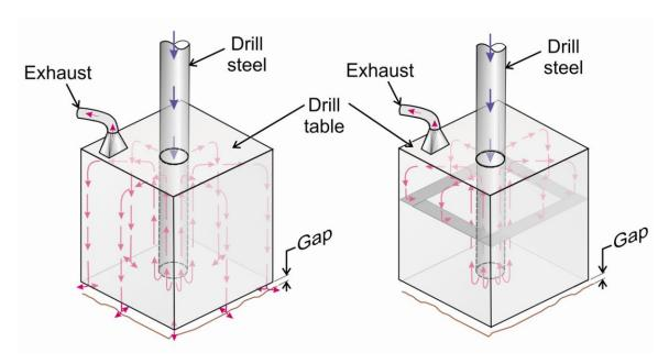
Figure 3.9. Qualitative models of airflow patterns underneath the shroud without the air-blocking shelf (left) and with the air-blocking shelf (right).
