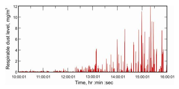
Figure 10.8. Respirable dust concentrations measured from haul road after water application occurred at 10:00 a.m. [Organiscak and Reed 2004]
