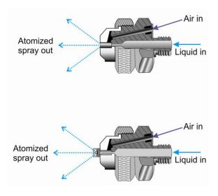
Figure 2.4. Typical internal mix nozzle (top) and external mix nozzle (bottom).
