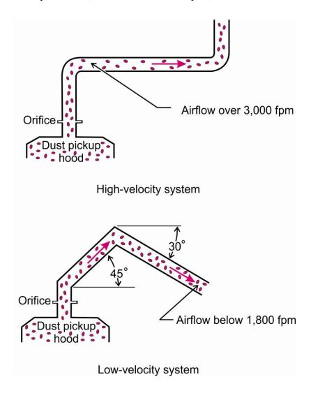
Figure 1.9. Schematics of high- and low-velocity systems.
