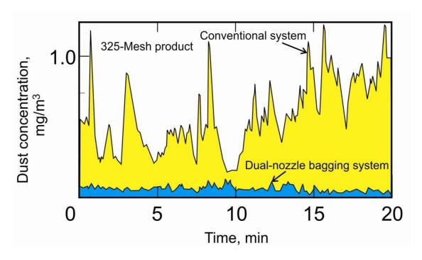
Figure 6.11. Bag operator's dust exposure with and without the use of a dual-nozzle bagging system.
