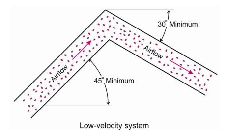
Figure 1.11. Duct design angles for low-velocity systems.
