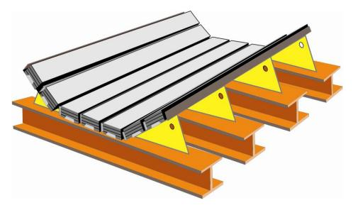
Figure 5.8. Depiction of an impact cradle with underlying rubber layers.
