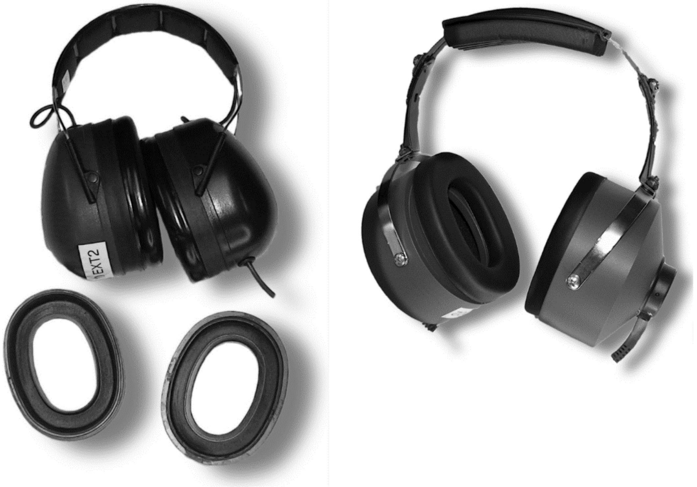
Figure 1. Headphones used with HPD Well-Fit. On the left are the modified Sennheiser HDA-200 headphones with spacers shown below. On the right are the Fit-Check headphones.
