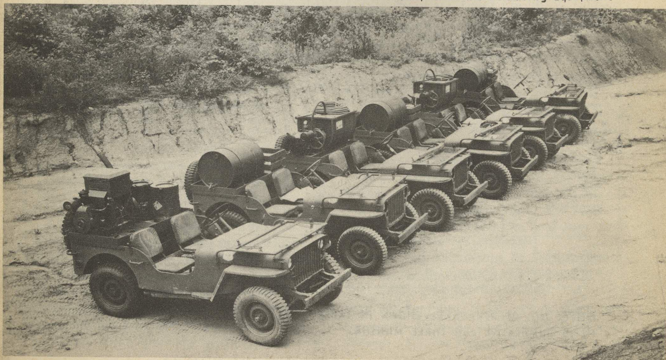
MCWA Jeeps Outfitted with Power Dusters and Oilers and Hand Oiling Equipment
