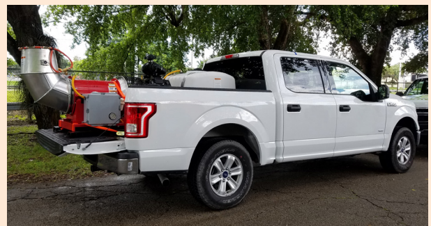
Mosquito control truck used for spraying larvicides
