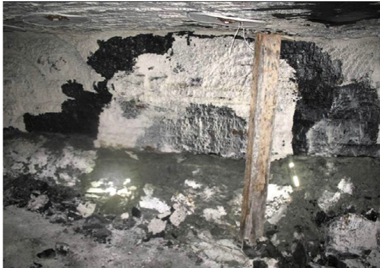
Fig. 15. Large slab formed as result of a thick clay band squeeze at mine USR 9.
