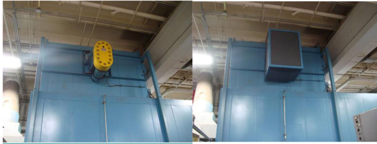
Figure 2. Noise control: Drum slitting and disc converting Controls Implemented: Acoustical enclosures installed around blower motors Direct Costs: $600
