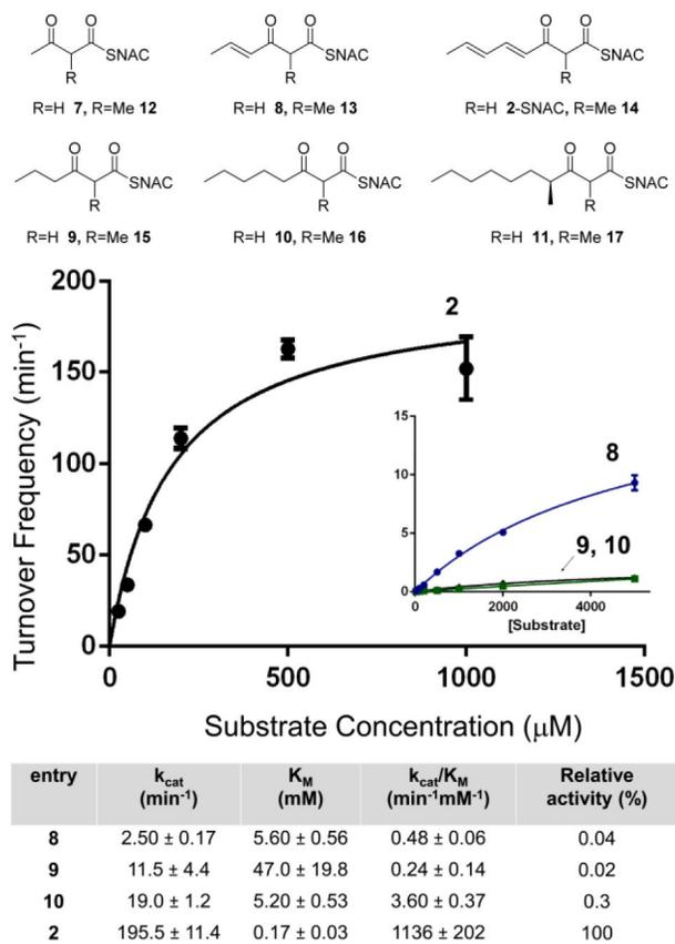
**Figure 2.** Full kinetic analysis of LovB MT domain towards different  $\beta$ -ketoacyl-SNAC substrates. **2** is the natural tetraketide substrate based on DML structure. **8** is the on-pathway triketide substrate of LovB. No reaction towards diketide **7** or pentaketide **11** was observed.
