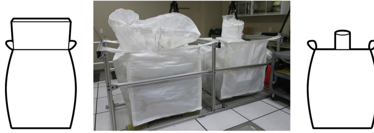
Fig. 1. Type of bags used; drawing of duffle (left), lab setup of duffle and spout, and drawing of spout (right).
