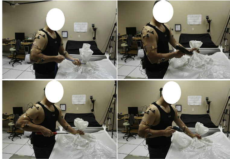
Fig. 4. Example of participant sealing the spout bag with the B-lock (top left), pneumatic cable tie gun (top right), pull twist tool (bottom left), screwdriver hook (bottom right).
