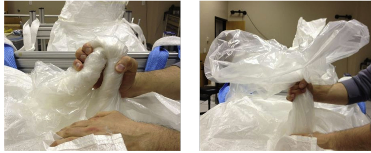
Fig. 2. Bag closing methods; snaking (left), flowering (right).
