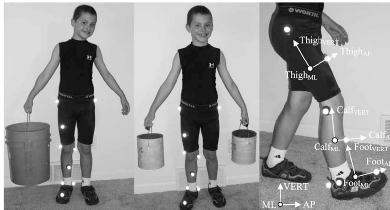
Figure 1. Representative eight-year-old child with reflective marker set. Left—unilateral large bucket carrying. Center—bilateral small bucket carrying. Right—segment and global coordinate systems.
