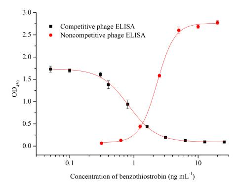
Fig. 2. Standard curves for benzothiostrobin by competitive and noncompetitive phage ELISAs. Serial dilutions of benzothiostrobin standard were mixed with phage-displayed peptides in optimized buffer, then  $100~\mu L$  of the mixtures were added to the antibody-coated wells. Each point represents the mean value of three replicates.
