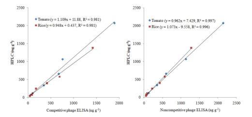
Fig. 3. Correlations between the phage ELISAs and HPLC for the samples containing incurred residues. Fourteen tomato and rice samples obtained from fields treated with benzothiostrobin were detected by competitive phage ELISA, noncompetitive phage ELISA and HPLC. The equation of the line and correlation coefficient obtained from linear regression of the combined phage ELISAs and HPLC data for benzothiostrobin in tomato or rice samples is shown.
