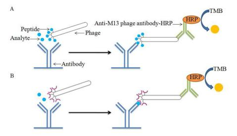
Fig. 1. Schematic diagram of competitive phage ELISA (A) and noncompetitive phage ELISA (B). The 96-well ELISA plate was coated with 1.0  $\mu$ g well<sup>-1</sup> benzothiostrobin antibody. Then 50  $\mu$ L of phage and 50  $\mu$ L of PBS with or without benzothiostrobin were added to the wells. A 1:5000 dilution of M13 phage antibody–HRP was used for the detection of bound phage.
