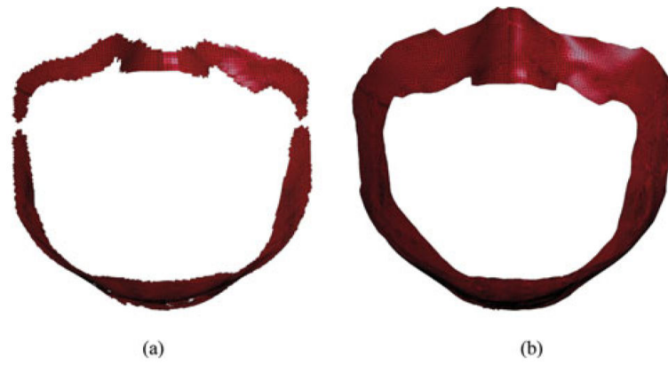
FIGURE 4. Contact area (a) the medium headform/one-size N95 FFR, (b) the medium headform/all fitted N95 FFRs. (color figure available online)
