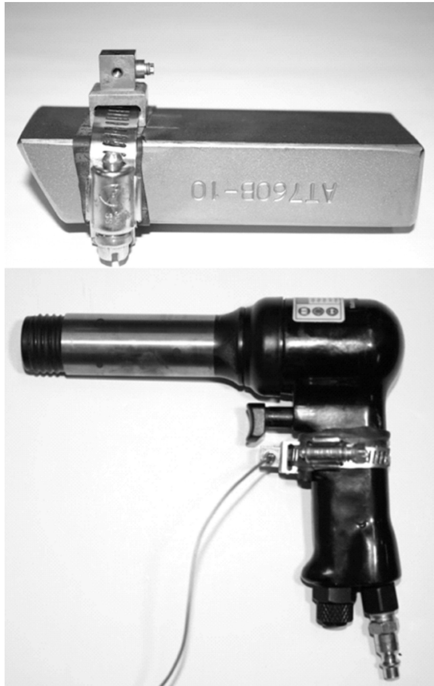
Figure 4. The accelerometer mounting technique. Synthetic rubber was used as a mechanical filter on each bucking bar to prevent DC shifts in the acceleration measurements. As can be seen in Fig. 3, electrical tape was wrapped around the accelerometer and clamp to prevent hand contact with sharp edges. This same technique was used to mount the accelerometer on the handle of the riveting hammer.
