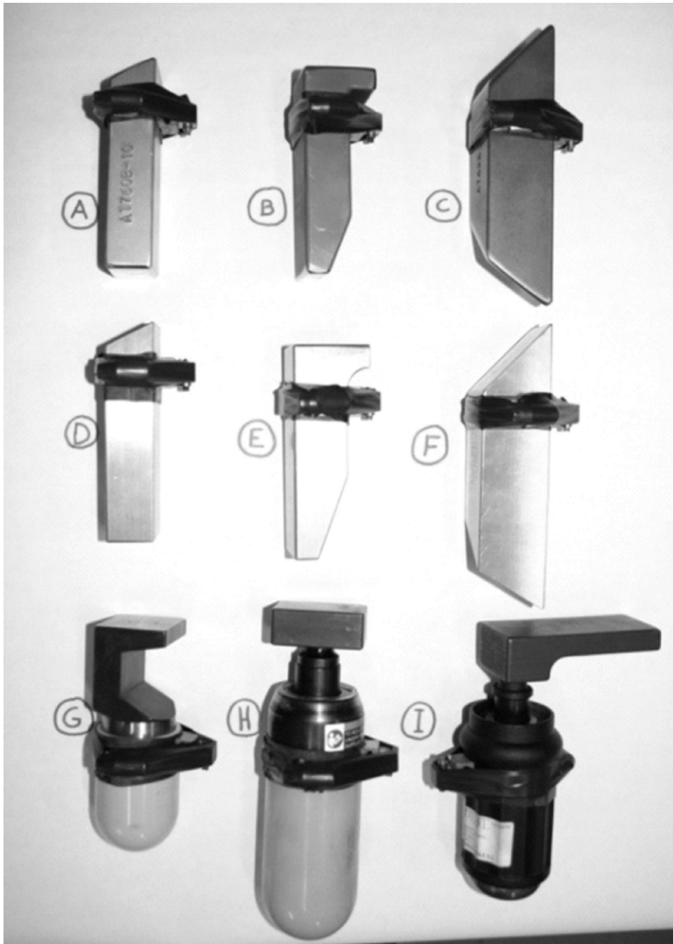
Figure 3. The nine bucking bars shown with tri-axial accelerometers mounted.
