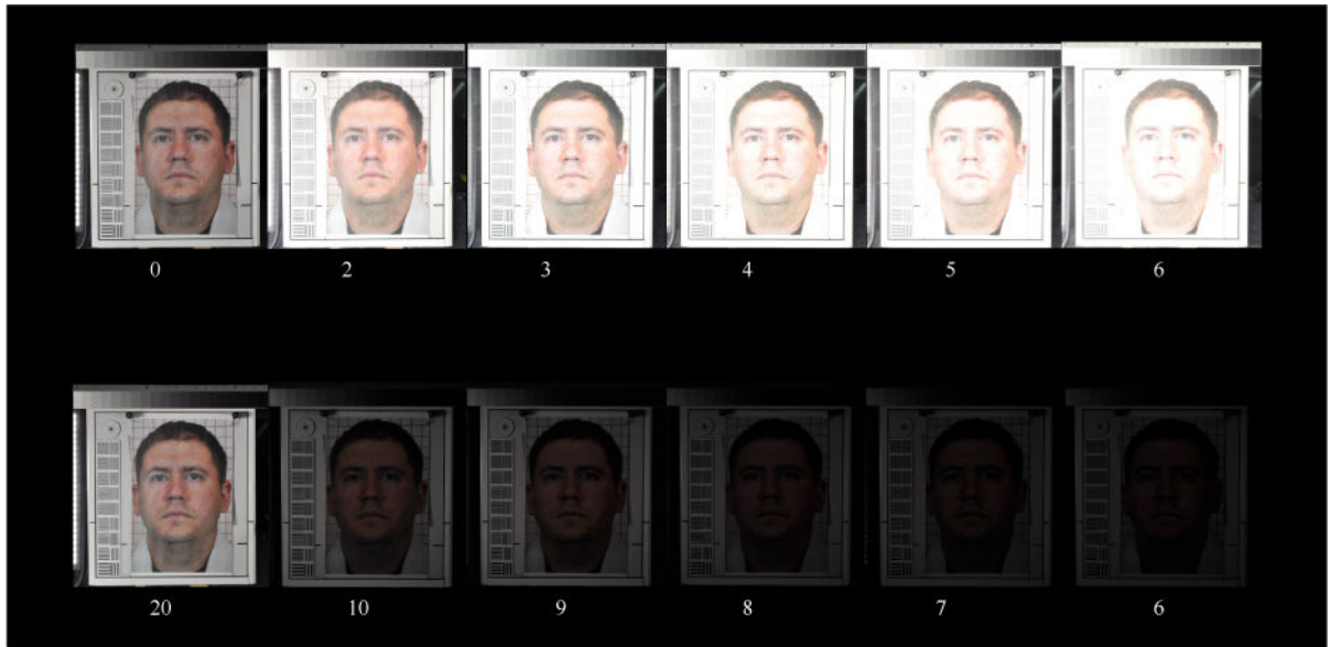
Figure 5. Six facial photos with different DRH (first row) with the number of washed-out gray steps, and six facial photos with different DRS (second row) with the number of recognizable gray steps.
