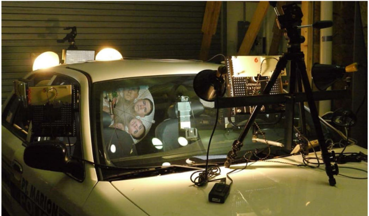
Figure 2. Four light conditions in each of the three taxicab seats were reconstructed in a simulated taxicab with seven white LED light panels and four incandescent light bulbs.
