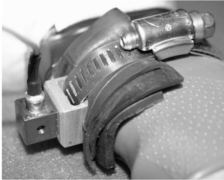
Fig. 3. Layers of synthetic rubber were used as a mechanical filter on each tool to prevent DC shifts in the acceleration measurements.
