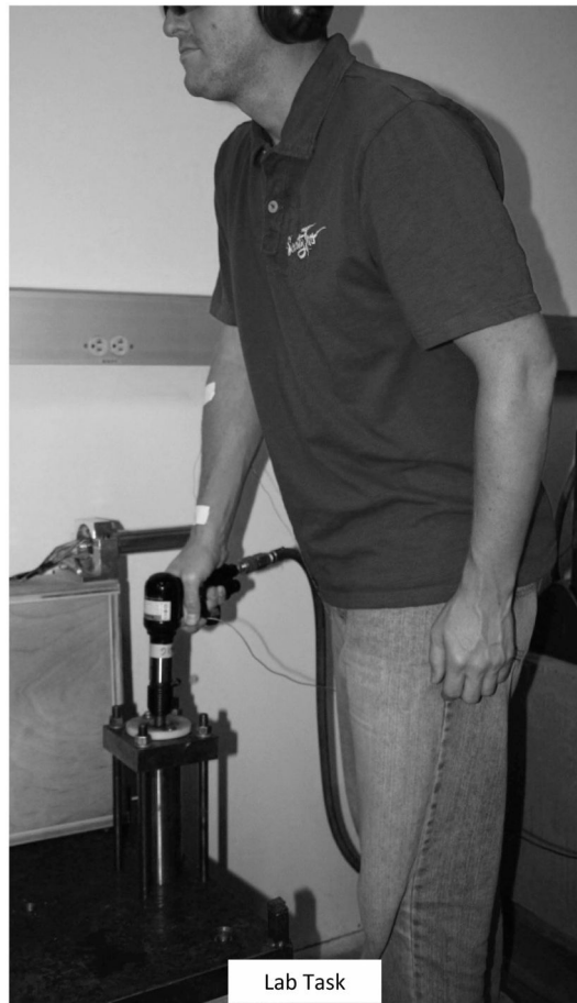
Fig. 4. The posture used in the laboratory portion of the study. The tool operators stood on a force plate and applied a downward pushing force (feed force) on the tool handle. The tool operator maintained the specified feed force ( 100 \pm 20 N) by monitoring the force displayed as a strip chart on a computer monitor placed directly in front of the operator.
