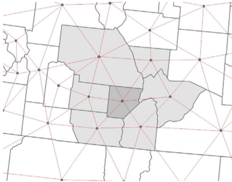
Fig. 1. Example of Delaunay triangulation. Counties in light gray are considered neighbors of the county shaded dark gray.
