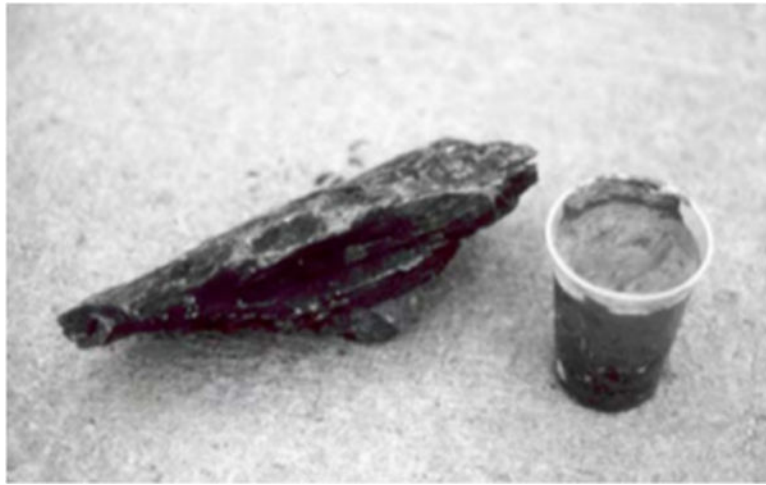
Fig. 3. The effect of water on a moisture-sensitive shale (from Mark and Molinda 2007)
