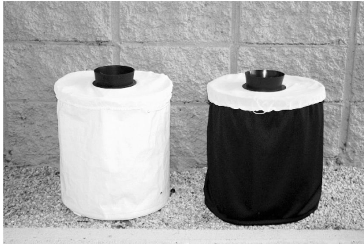
Fig. 1. Original BG-Sentinel trap (white; left) and modified BG-Sentinel trap, showing the black outer cover (right).
