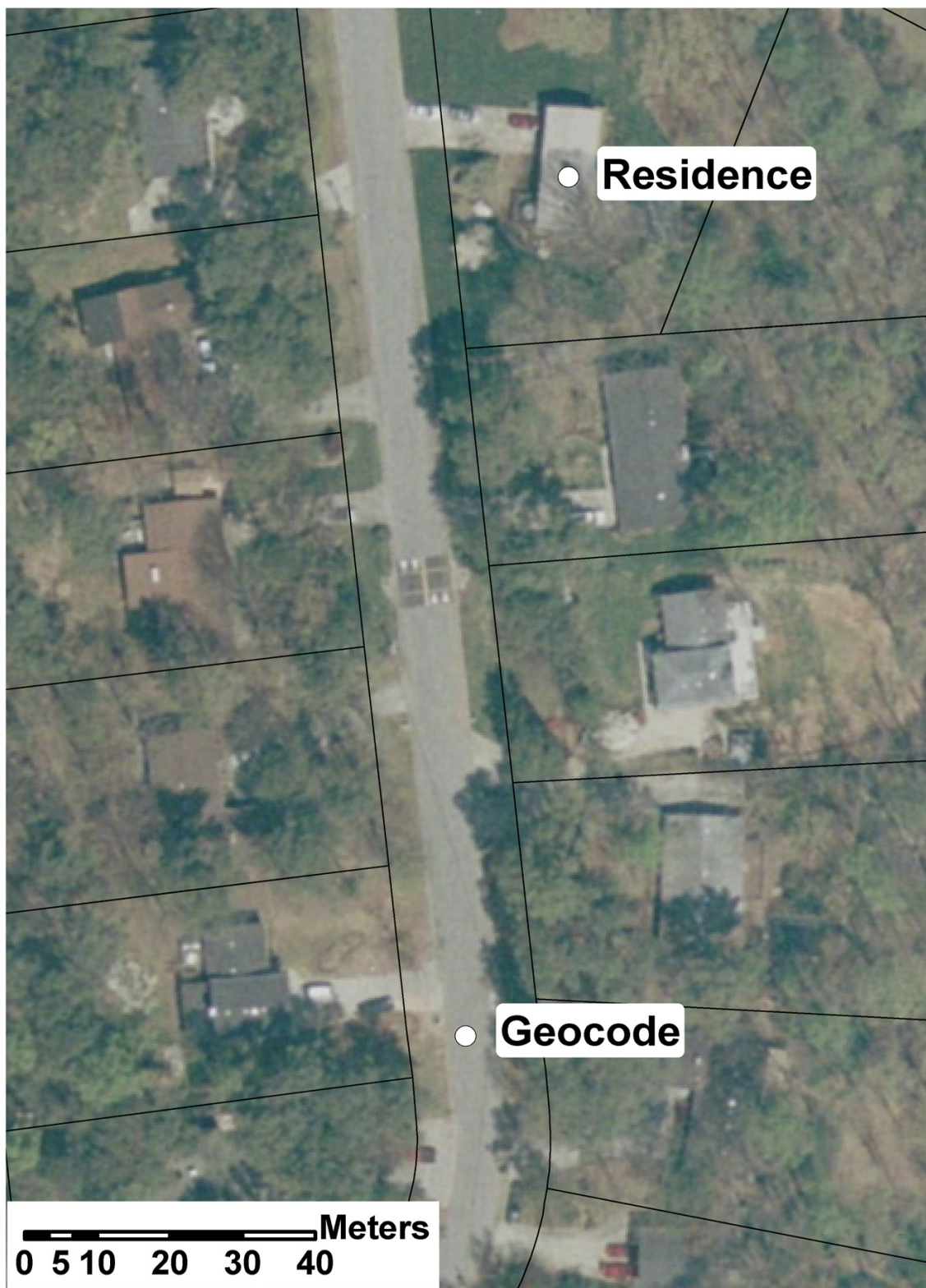
Figure 1 Tax Parcel Data Overlain on Orthoimagery. The distance between the geocode and the residence (gold standard) is the "location error" for the address.
