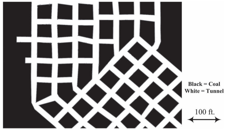
Figure 10. Map of mining area showing room-and-pillar layout.
