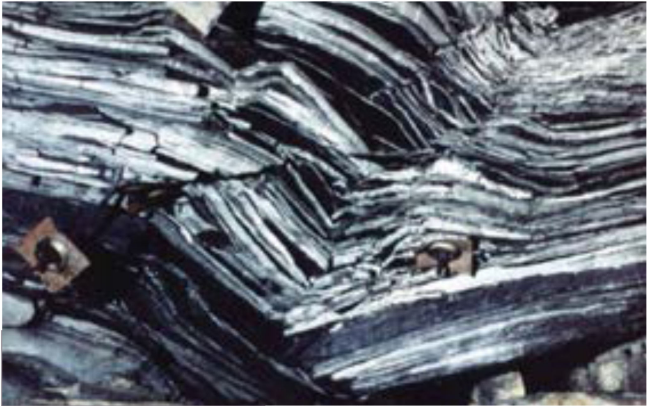
Photo 1. Failure of laminated roof layers in a coal mine.
