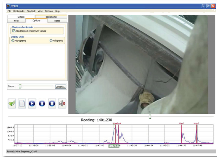
Figure 3. Screenshot of miner using manual scraper to bypass the screening process until product was dry.
