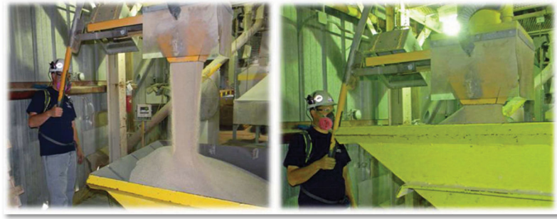
Figure 4. FIBC loading operator performing a load-out task with dumpster on floor (L) and a modified setup with dumpster raised (R).
