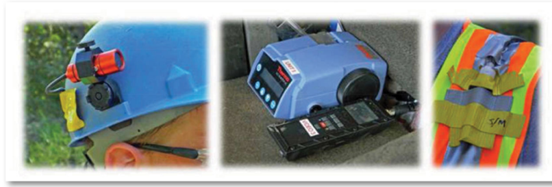
Figure 1. Helmet-Cam setup showing video camera lens on a miner's hardhat, the digital video recording portion of the video camera and pDR-1500 dust monitor, and the 10-mm cyclone.
