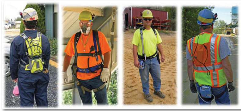
Figure 2. Various options to house the Helmet-Cam system: backpack, two types of miners' safety belts and safety vest.
