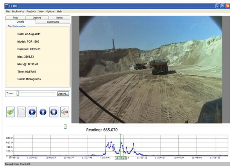
Figure 5. Screenshot of EVADE user’s screen. The video is in the top right corner and the respirable dust control graph appears along the bottom of the screen. Each blue dot on the graph represents a two-second respirable dust measurement. This Helmet-Cam unit was inside the enclosed cab of a haul truck.
