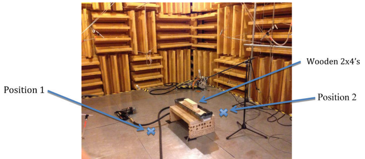
Fig. 4. Framing nailer test setup. Wooden two-2x4s are stacked in the sand box to receive the nails. The framing nailer operator made approximately ten measurements in position 1 and ten measurements in position 2.
