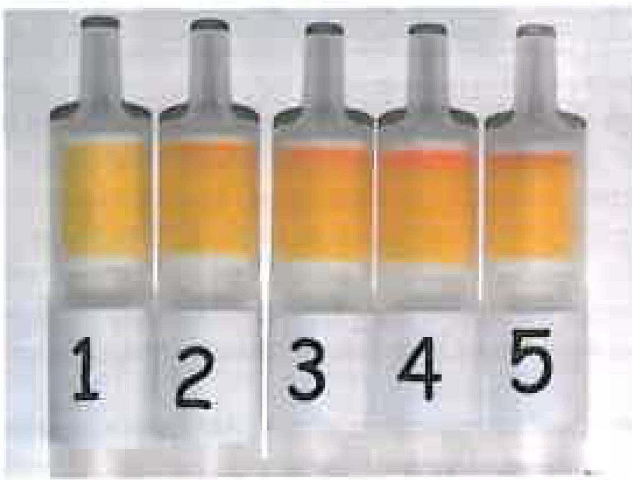
Fig. 7. Colored bands of OPA derivative on S10 LpDNPH samplers. Sampler 1 is a blank sampler and exhibits DNPH-coated silica in a bright yellow color. Samplers 2, 3, and 4 exhibit orange or red-orange bands after the collection of 12, 36 and 120 \mu\text{g} of OPA, respectively, in mixtures of condensation aerosol and vapor at 60% relative humidity from a glass U-tube partially immersed in an oil bath at 120 ^{\circ}\text{C} . Sampler 5 exhibits a brown band after collection of 43 \mu\text{g} of OPA vapor at 23% relative humidity from the OPA generation system.
