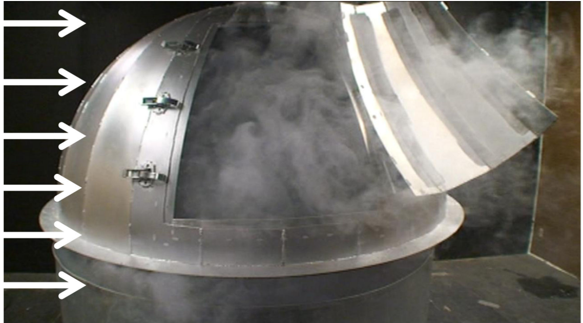
FIGURE 10b. Dome hood with 114-mm gap (at 5.66 m 3 /min and 30 m/min cross draft). Note: White arrows reflect direction of airflow from industrial floor fan.
