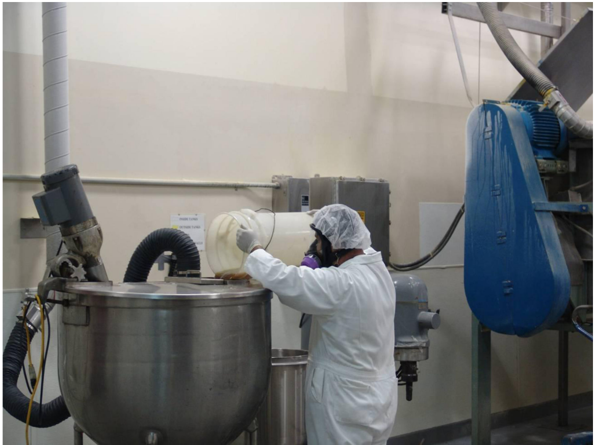
FIGURE 1. Flavoring ingredients manually added to the mixing tank with a ventilated lid through an access port at a flavorings plant
