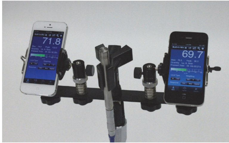
Figure 1. The SoundMeter app on the iPhone 5 (left) and iPhone 4S (right) compared to ½” Larson-Davis 2559 random incidence type 1 microphone (center).
