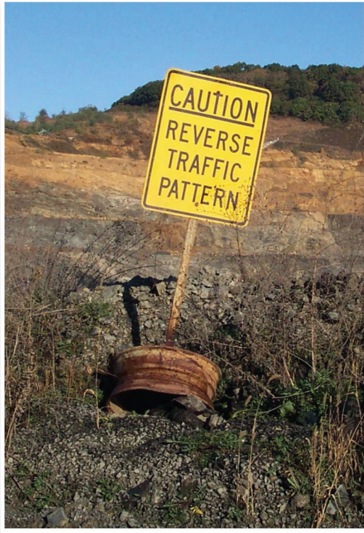
Figure 2. Example of a sign used at surface mine site to warn operators of haul road traffic pattern.
