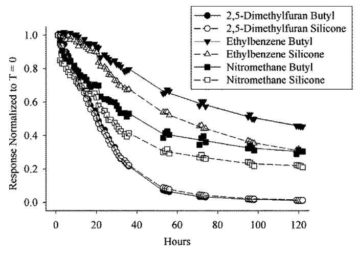
**Figure 1.** Change in absolute response for ethylbenzene, 2,5-dimethylfuran, and nitromethane using bags fitted with butyl Orings, shown as filled symbols with a solid line, and silicone O-rings, shown as open symbols with a dashed line, for a 3R4F research cigarette vapor phase sample analyzed over a 5 day period.
