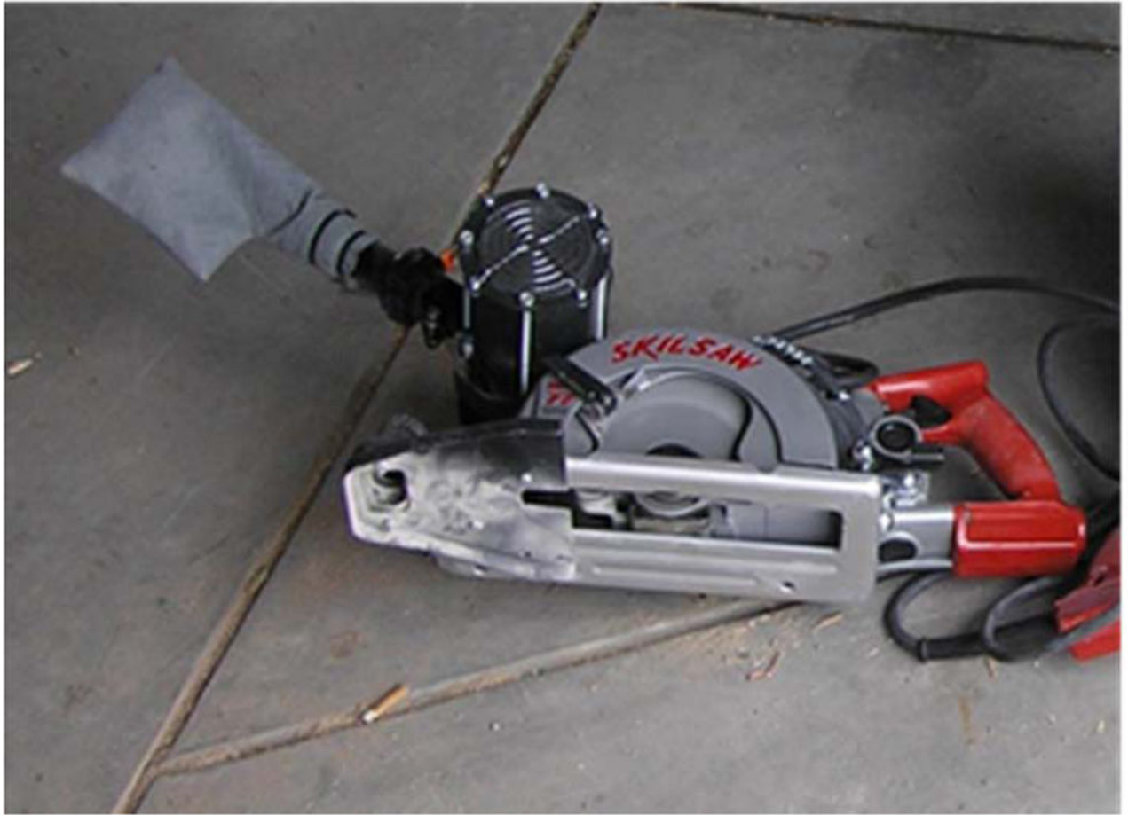
Figure 3. Circular saw with aftermarket local exhaust ventilation
